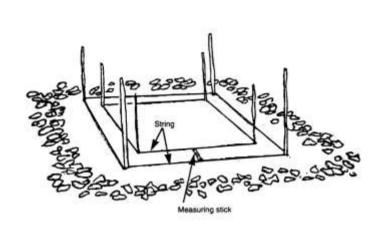
Figure 1: Marking out for a square building
