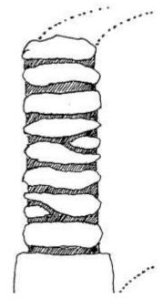
Figure 4: The foundation layer is wider than the wall
